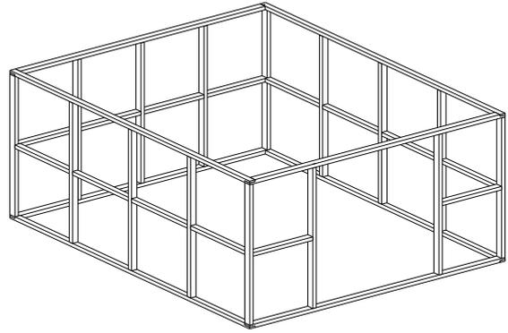
**Step 5:** Position middle Jack Stud, centrally on End Wall Top Plates and nail in place. Nail remaining Jack Studs in. Position middle Ridge Beam to Jack Stud and skew-nail in place using two 75mm nails each end. Pre-drilling holes before nailing will prevent timber from splitting.
