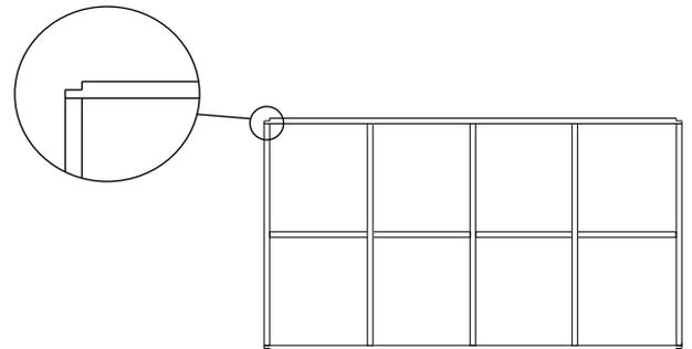
**Step 2: Front Wall:** Select one 3.380m Base Plate (Green), one 3.380m Top Plate (Red), four Studs (Yellow) and two .785m Nogs. Nail studs to each end of Plates. Nail in remaining two studs using .785m Nogs to get correct position. Position Nogs .883m below Top Plate and nail in place.
