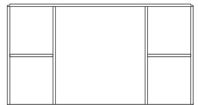
**Step 3: End Wall:** Select one 3.380m Base Plate (Green), one 3.380m Top Plate (Red), three Studs (Yellow) and two .787m Nogs. Lay out Plates and one Stud on a flat surface and nail Stud centrally between Plates. Nail remaining Studs to Plates using .787m Nogs to get the correct position. Position Nogs .883m below Top Plate and nail in place. Repeat with second End Frame.
