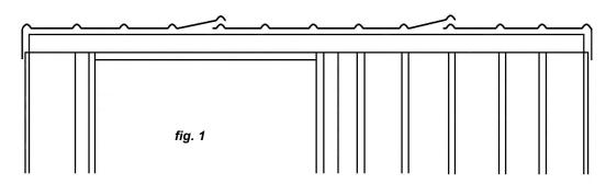
**Step 1: Note:** Condensation can form on the under side of shed roof. If building paper is required, fit now. Building paper will need to be supported by netting or roofing twine.
