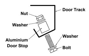
Step 4: Clean out ALL drill filings. Also make sure the Wheels are cleaned of drill filings. Re-hang Door, then insert door stops into the pre drilled holes at end of tracks as shown in diagram. Tighten with two spanners.
