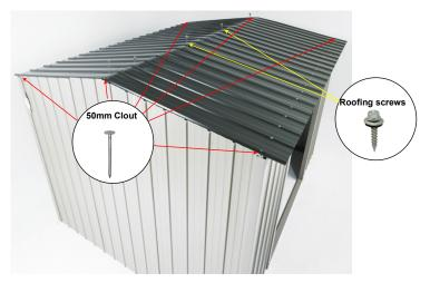
Step 3: Starting from the left hand end, centralize Roof on Ridge Beam. Ensure Roof is tight against end Wall Sheets, predrill then nail one 50mm Clout through Rib into the Ridge Beam. At the back, line up Ribs on the Roof Sheet with the Ribs on Wall Sheet. Using one 50mm Clout, nail through Rib into Back Top Plate. Repeat at the front.
