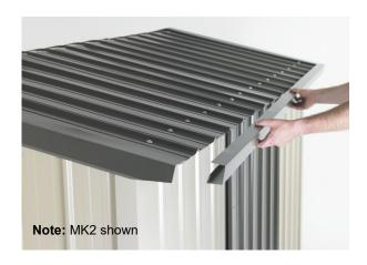
**Step 1:** Position Barge Flashing (102) on gable ends. Position a Spouting (A103) and rivet to the Barge Flashing at each end. Repeat with other Spouting.
