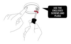
Once the mounting base is installed, attach the alarm by twisting clockwise until it clicks. If the battery is either missing or inserted incorrectly, or the switch is in 'Link Mode', the heat alarm will not be able to click into the mounting base.
