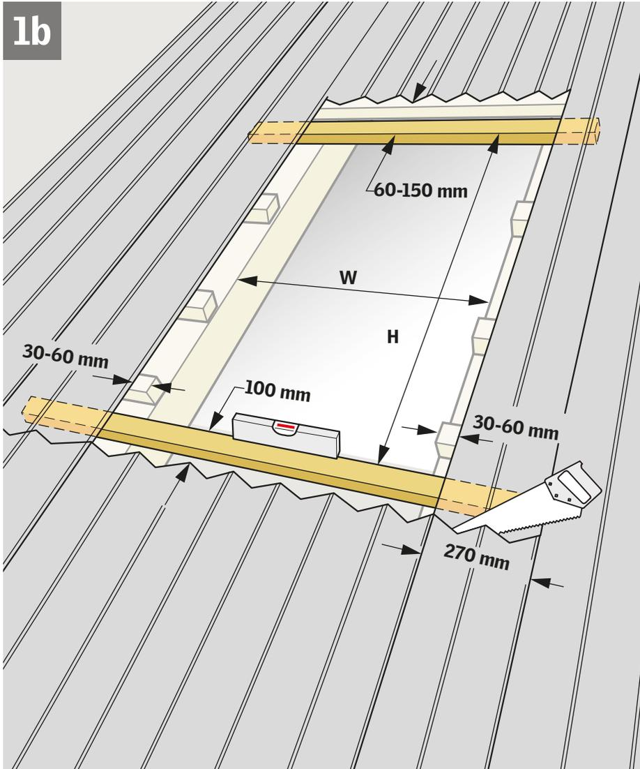
**ENGLISH: Existing metal sheet roofing with flashing EDW**
