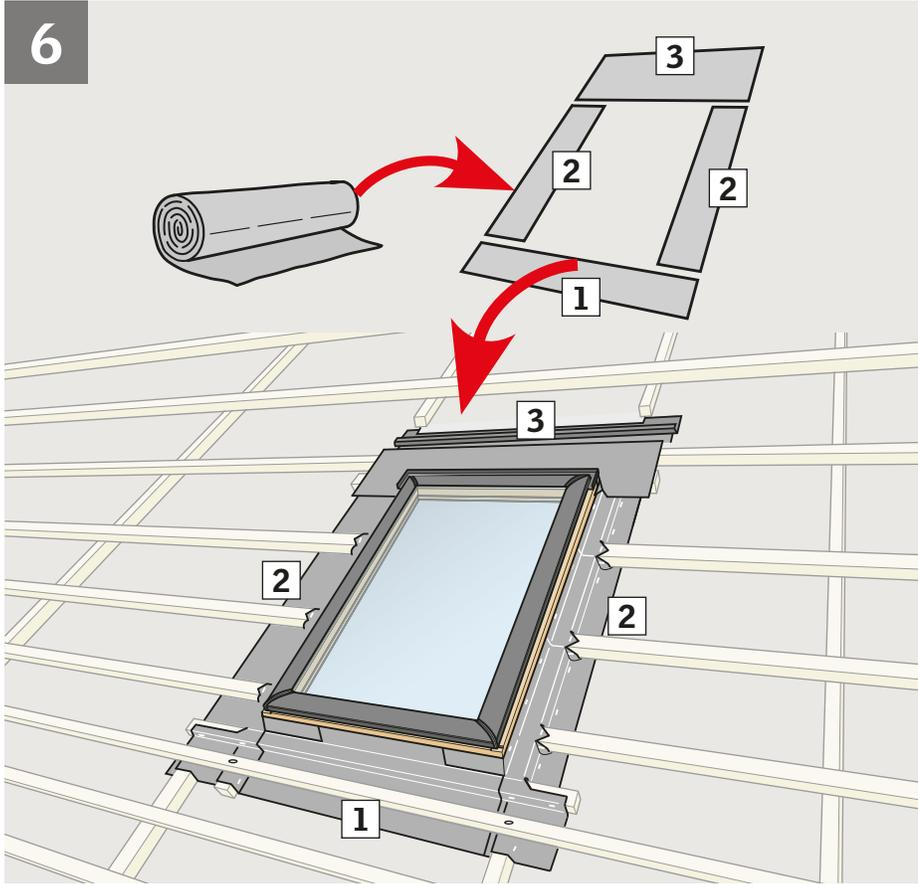
**ENGLISH:** If roofing underlayment is used: Dress roofing underlayment up around all four sides of the frame. Roof with counter battens shown for illustration purpose.
