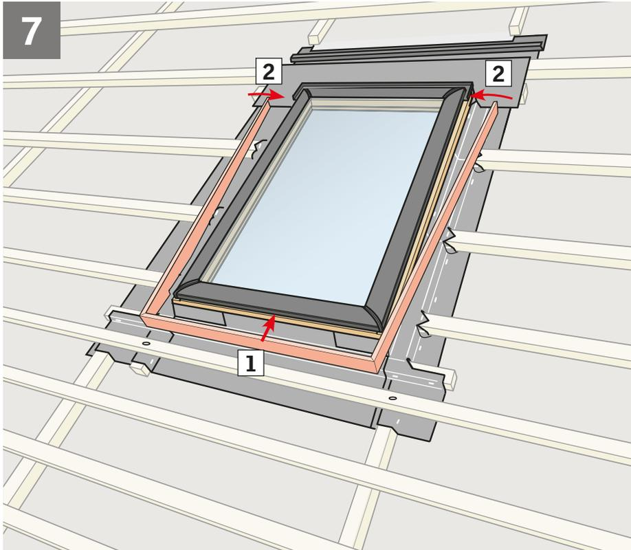
**ENGLISH:** If flashing is not to be installed immediately, replace the cladding parts starting at the bottom. Interlock side frame claddings with bottom frame cladding as shown. Secure the claddings with the original screws.
