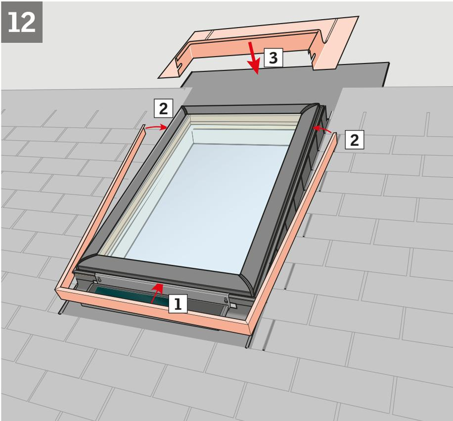
**ENGLISH:** Reinstall cladding (1), (2) and continue installation of flashing (3) as shown in the instructions provided with the flashing.
