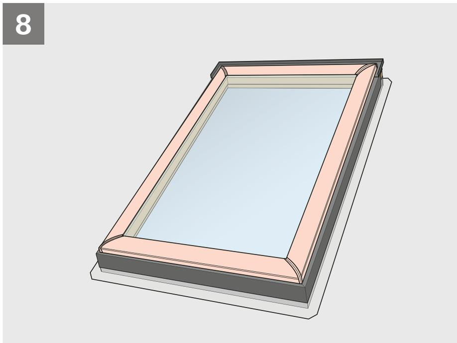
**ENGLISH: Caution:** Removal of sash during installation of the skylight is not recommended. If sash is removed, test and check that it is properly attached at the top and bottom of the skylight frame. If working from an interior room, close the skylight completely. To verify that it is properly attached, carefully push outward on the sash. If working from the roof, close the skylight completely. To verify that it is properly attached, carefully try to lift the sash away from the skylight.
