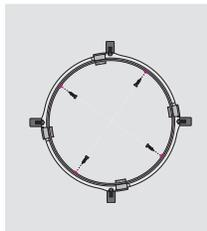
**ENGLISH:** Secure tunnel assembly to ceiling ring with four of the 3/8" (10 mm) screws provided.
