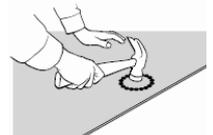
Tap carefully to avoid damage to sheets, ensuring that the sheet edges are properly supported.
