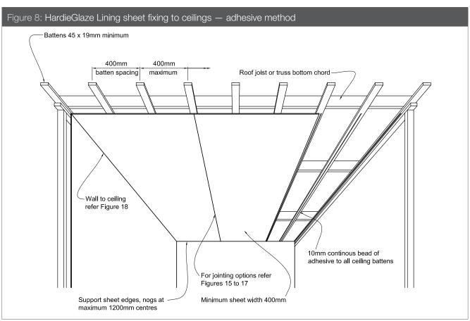
Note: This method requires the sheets to be fully braced temporarily while the adhesive cures (refer Figure 11). Bracing member should be aligned with the framing behind HardieGlaze Lining.
