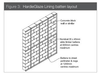
Note: Steel battens 72mm wide x 23mm deep x 0.55mm thick, with a minimum bearing surface of 38mm and with minimum 275g/m<sup>2</sup> zinc coating, can also be used.
