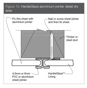
When using a cap mould, cut the vertical jointer shorter to suit.
