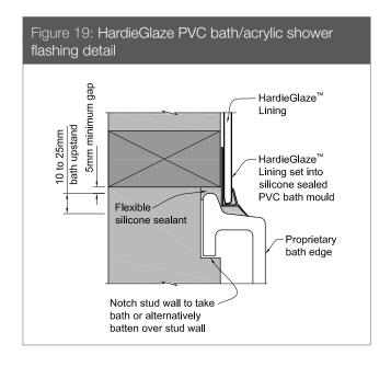
Note: Seal bottom edge and 100mm up back of sheet with Dulux 1 Step, Dulux Acraprime 501/1 or similar.
