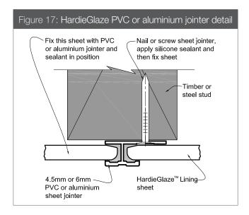
Note: For showers and similar wet areas the PVC or aluminium jointer must be silicone-sealant filled. External and internal corners and cap moulds must also be silicone filled in these wet areas.
