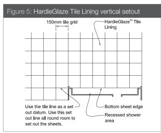
Note: Sheet set-out is important in visible areas of the room. Use full sheets in these areas and save part sheets for less visible corners. If tile pattern set out allows use a factory finished bottom edge in wet areas. Seal bottom edge and 100mm up back of sheet with Dulux 1 Step, Dulux Acraprime 501/1 or similar.
