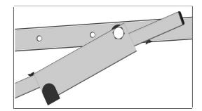
The smaller Addaline frame is raised and lowered, by manually securing the wire Braces into the Side Arm's larger punched holes.
